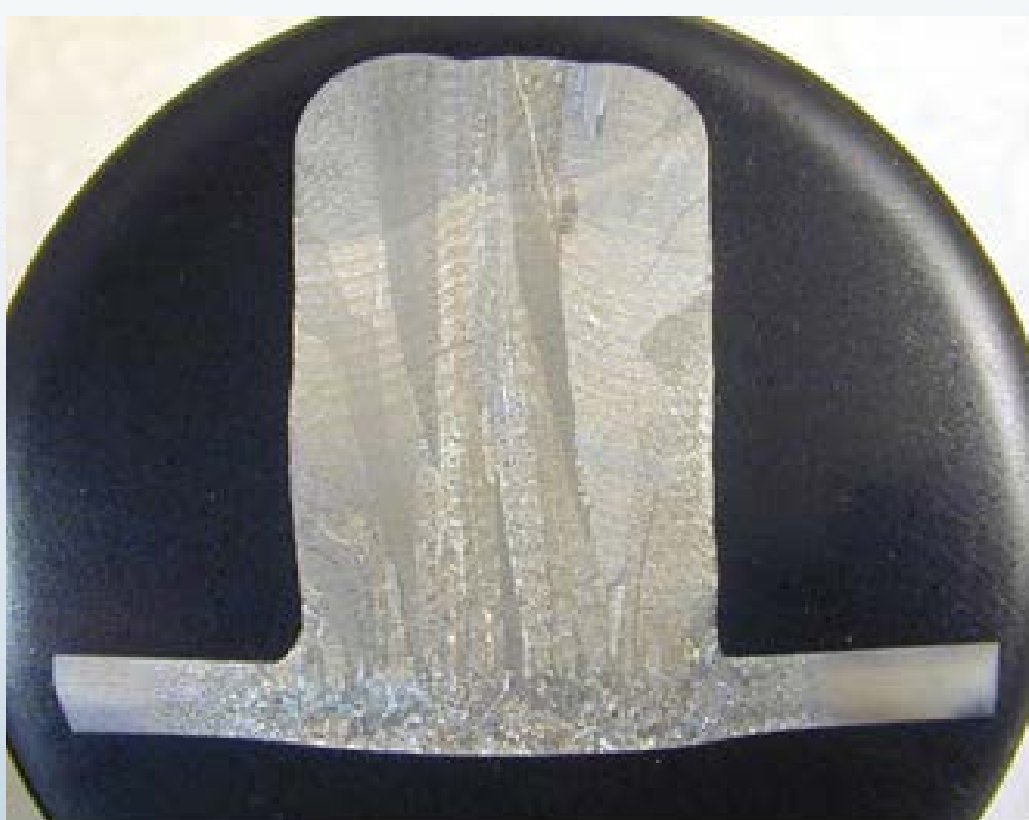
Additive manufactured Ti-64 showing microstructure variations.
