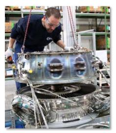
GKNs turbine structure – engine test at MTU in Germany 2015 (HDL – hydroformning)
