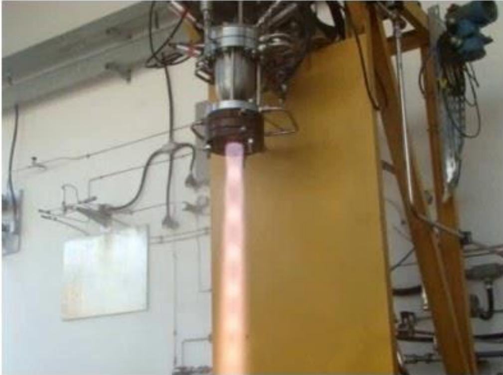
**Testbed for liquid propulsion**
