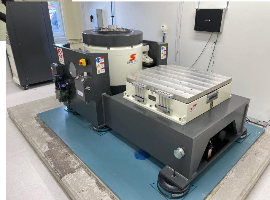
New vibration testing facility
